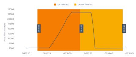
Our tests have confirmed the rapid and efficient responsiveness of DC EV chargers within the Emulate and eMabler systems to energy management commands, both for scaling up and down.
